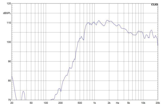
Frequency response measured at 90°x50° horn
