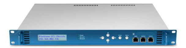
HP714D 4 IN 1 IRD is a integrated receiving device which can receive the transmission stream from tuners. This 4 in 1 IRD is equipped with CAMs/CIs and can decrypt 4 tuners input programs. It support 4 DVB-C/S2/T2 Tuner inputs and IP(4\*MPTS&64\*SPTS) output throught dual gigabit ethernet and 4 ASI output.
