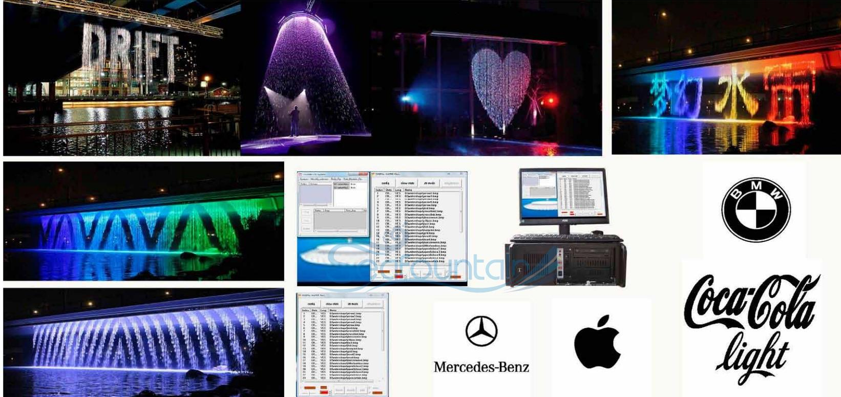
❖ **Digital Water Curtain** is special water curtain in the fountain industry. The computer system can convert the designed patterns into different control signal for the solenoid valves which can command the timing of water falls, then water curtain can form the patterns designed.
