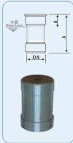
Mist spray nozzle can produce aerosol effect under high pressure of pump. With little noises and small water consumption, mist spray nozzle is normally installed around sculptures and applied together with Musical Dancing Fountain or Program Control Fountain.
